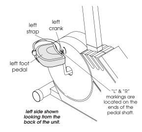
Figure 7 - Install Foot Pedals
